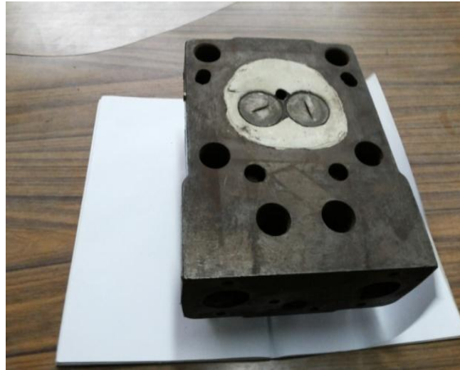
Plate 1: Photographic View of the Ceramic Coated Cylinder Head
